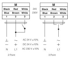
↑ Connect via safety isolating transformer
