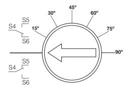
Switch **(a)** factory-fixed at 5° Switch **(b)** adjustable 0°...90°
