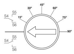
Switch **(a)** factory-fixed at 5° Switch **(b)** adjustable 0°...90°
