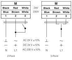
↑ Connect via safety isolating transformer
