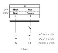
↑ Connect via safety isolating transformer
