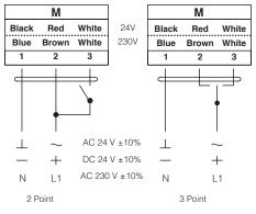
↑ Connect via safety isolating transformer
