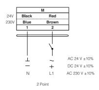
↑ Connect via safety isolating transformer
