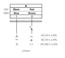
A Connect via safety isolating transformer
